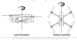
Tips: It's a must to have the right compass adjustment first each time you start the drone. or it can't work normally.
