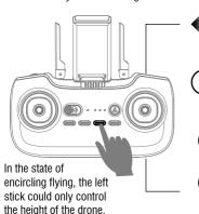
Turn left, the drone flies clockwise: Move further, the flying speed will become faster
