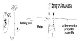
Remove propeller components in serial order. Operation in the opposite direction dring installation. The propeller is divided into AB, corresponding to the letter on the folding arm. Please make sure it is installed correctly,otherwise it cannot fly.
