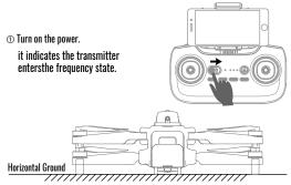
The drone is placed on the horizontal ground, long press the power button for 3 seconds to turn on, the front and rear navigation lights cycle flashing, indicating that the frequency alignment is successful to enter the GPS start search state.
